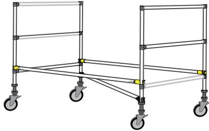
**4** Attach the Plan Brace (Black) to diagonally opposite uprights below the first rung. Check to see if the scaffold is square. Ensure that the scaffold is level by using the adjustable nuts on the castors.
