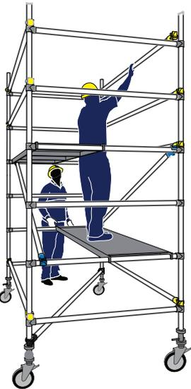
**7** Install a temporary platform between the two Base Frames at approximately 1.0m high. Then install the Trapdoor Platform between the two frames at approximately 2.0m high, offset from the first platform.
